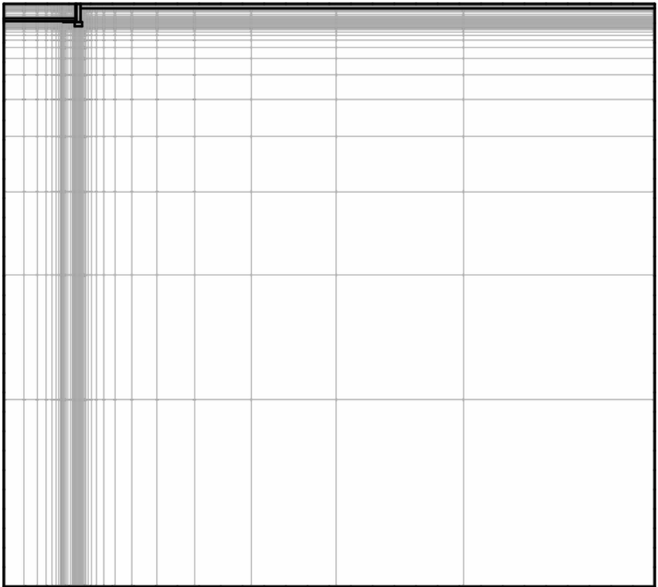
Example generated discretisation of full domain
